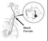
The steel tubes are meant to substitute relatively straight areas of cable routing, to eliminate friction and compression. DO NOT BEND TUBES!!
