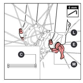
Close the locking device (**M**) and tighten both screws (**L**) with a 6mm Allen wrench.
