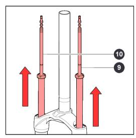
· Pull the crown-stanchion unit (3) off the arch-slider assembly (4).
