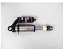
B – 3 Way Swinger Coil Shock, No Hardware, No Coil B – 4 & 6 Way Swinger Coil Shock, No Hardware, No Coil
