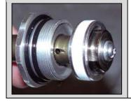
25. Reinstall piston, shim stacks and the SPV valve on to the damper shaft, tighten bolt to 80inlbs. Line the damper cap up so that the inner end of the cap is lined up with the edge of the bleed hole in the damper shaft. Fill the damper body with oil.
