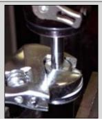
5. Remove the Damper Cap/ Air Piston Cap from the damper body. Using an adjustable wrench or 14mm wrench. Pull damper shaft assembly from the damper body. Pour out the oil that is in the damper body.
