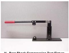
H - Rear Shock Compression Test Fixture
