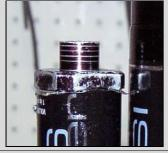
15. Make sure that the IFP Positioning Tool is in its shortest position; Screw it down into the reservoir pushing the IFP into the bore. If you are rebuilding a Revox shock, be sure that you fit the IFP extension (P/N \*\*-\*\*\*\*) to the Positioning tool before installing it into the reservoir.
