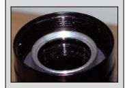
24. Install the air piston into the air can and push it all the way down until it seats fully on to the top of the damper body. There should be no space between the top of the damper body and the bottom of the air piston.
