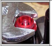
21. Remove the IFP tool from the reservoir and install the Volume control assembly. Torque the assembly to 100inlbs (11Nm). Turn the control to the open position, this is where the indicator is in the number 1 position, this allows the entire volume control to be pressurized. On Swinger and Revox SPV shocks, charge the IFP to 120psi. For the shim versions of the Revox and Swinger coil the charge pressure is 150psi. For the metal shocks the IFP charge pressure is 250psi.
