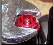
2. Remove the No Tools Volume adjust by unscrewing it counter clockwise. There is no need to disassembly the assembly any further as there are no parts to wear in the no tools adjuster.
