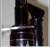
32. Pull the air can up and screw the top cap down. Clamp the top cap in the vise and using a 39mm wrench torque the air can to 80 inlbs (9Nm)
