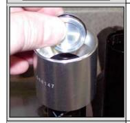
14. Install the bleed bowl, and fill the reservoir and bowl with 5wt shock fluid. Install the IFP by lowering it into the fluid vertically so no air is trapped in the cavity if the piston. Turn the piston 90 degrees and push it into the reservoir past the threads. Remove the oil above the piston. Remove the bleed bowl.
