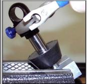
20. Clamp the damper shaft in a vise using the 12mm shaft blocks. Apply blue Loctite to the threads of the damper shaft. Screw on the damper cap and to torque it to 110inlbs. (12 Nm)
