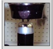
23. Insert the air can installation tool into the damper body. Slide the air can over the tool and on to the damper body. Next install the top out bumper then remove the Installation tool.
