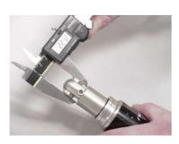
2. Measure mounting hole size. Current hardware is typically designed to accept a 6mm or 8mm fastener.
