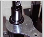
2. Remove the Air Can from the shock using a 39mm wrench or an adjustable wrench if it is an X3, if it is a Radium or S-Type you will need to use a strap wrench to remove the air can. It will unscrew in a counter-clockwise direction.
