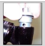
12. Secure the shock eyelet in a vise with the mounting hole for the intrinsic damper up. Fill the hole with oil and install the Intrinsic damping control unit. If it is an adjustable unit for an X6, be sure that the adjusters are turned out to the lowest settings
