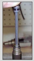
27. Insert the rebound preload spring and rebound needle into the damper shaft and then screw on the top cap. Using the top cap fully extend the damper shaft. Remove the top cap and the rebound needle.
