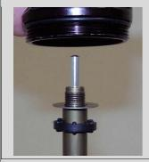
29. Reinstall the rebound needle, bottom out bumper, and the bottom out washer. Clean the tread of all oil residue.
