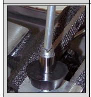
Reinstall the rebound needle, and bottom out bumper. Clean the tread of all oil residue.
