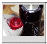
31. Remove the IFP tool from the reservoir and install the Volume control assembly. Torque the assembly to 100inlbs (11Nm). Turn the control to the open position, this is where the indicator is in the number 1 position, this allows the entire volume control to be pressurized. On Swinger X4 shocks charge the IFP to 125psi. For the Evolver shocks the SPV version is charged to 120psi and the shim version to 150psi. The charge pressure is 250psi on the Split shocks.
