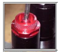
1. Turn the Volume adjuster so that it is in position. Release the air in the IFP chamber and remove the Schrader valve core.
