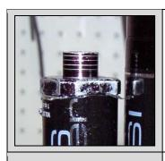
20. Make sure that the IFP Positioning Tool is in its shortest position; Screw it down into the reservoir pushing the IFP into the bore.
