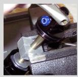
30. Clamp the damper shaft in a vise using the 12.5mm shaft blocks. Apply blue Loctite to the threads of the damper shaft. Screw on the damper cap and to torque it to 110inlbs. (12 Nm)
