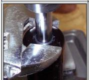
Make sure that the shock is full extended. Clamp the shock in a vise by the damper eyelet. Using a 28mm or an adjustable wrench, remove the damper cap and shaft from the shock by turning it counter-clockwise. Drain out as much fluid as possible after pulling the damper assembly out of the shock.
