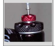
33. If applicable, install the detent springs, balls and knobs on the Intrinsic Adjuster. Make sure that the set screw on the high speed compression knob (black knob) is lined up with the pocket on the adjuster shaft before tightening it. Next install the red lox speed compression knob.
