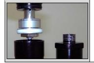
17. Insert the damper piston/shaft assembly into the damper body. Screw down the top cap and torque to 60-70inlbs. Make sure that the shaft isn't moving out as you do this.
