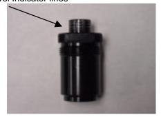
17. Under oil, screw in the IFP locating tool into the air reservoir body. This will press the IFP deeper into the reservoir body to the required depth.
