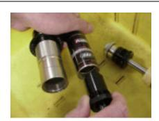
18. Under oil, screw in the damper assembly hand tight until damper cap is flush with the damper body.
