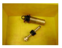
10. Remove assembly from the oil, keeping the open end of the damper shaft pointing up. Using soft jaws to protect the eyelet, clamp the reservoir eyelet and tighten the damper cap per Table 1.
