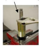
4. Using pliers, remove the rebound adjuster needle from end of the damper shaft.
