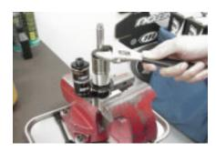
20. Holding the assembly over the oil container, Install rebound adjuster needle, pointed end first. Push until the needle oring seats in the damper shaft.
