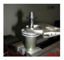
15. Clean the damper shaft threads with alcohol and install the rebound eyelet using 10mm soft jaws and red Loctite. Torque per Table 1.
