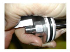
10. Immerse damper body and damper in oil to
