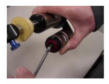
Unscrew air preload assembly and damper shaft assembly using an adjustable openend wrench.
