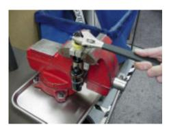
22. Remove the IFP location tool. Once the tool is removed DO NOT move the damper shaft
