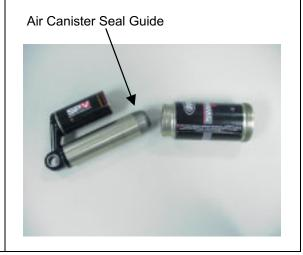
11. Grease inside of air canister and install air canister as shown. The seal end of the air piston is installed first.
