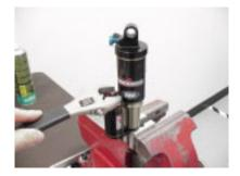
4. Using 10mm soft jaws, clamp the damper shaft and remove the eyelet as shown.
