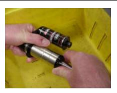
19. Remove the assembly from the oil, keeping the open end of the damper shaft pointing up. Using soft jaws to protect the eyelet, clamp the reservoir eyelet and tighten the damper cap per Table 1.
