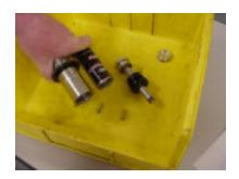
15. Under oil, insert the IFP into the air reservoir using the Swinger Air IFP removal tool. Only press the piston in just beyond the reservoir threads.
