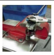
Clamp the damper body eyelet in a vise using soft jaws and remove the damper assembly by removing the air piston and damper assembly using an 18mm socket as shown.
