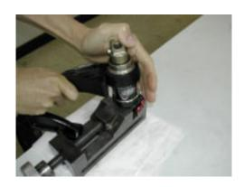
4. Using 10mm soft jaws, clamp the damper shaft and remove the eyelet as shown.
