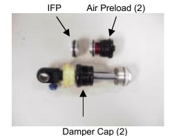
10. If oil was leaking from one of the high or low speed compression adjusters on a 6 Way Swinger, the adjusters should be replaced, <u>Do Not</u> remove unless a leak was detected. Remove the two 1.5mm set screws found on the backside of the reservoir forging. Remove the adjuster needles using a 3mm hex (Early Model Year 2004) or 2mm hex (Late Model Year 2004), Pour a small amount of damping oil in each hole prior to replacing the needles.
