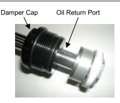
14. Place damper body, damper shaft assembly and IFP into damping oil. With the open end of the damper body pointing slightly up, gently tap the body to dislodge any entrapped air and set down. Do the same with the damper assembly, pointing the damper shaft slightly up to remove any air bubbles.
