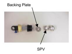
Separate the two halves as shown. Inspect the two seals for signs of damage. Grease seal surfaces and reassemble.
