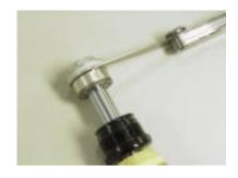
Remove IFP (Internal Floating Piston) using a shock pump to pressurize the damper body. Point the damper body <u>away</u> from you as you pressurize the body and expel the IFP
