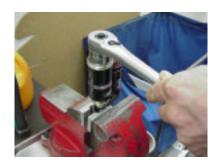
6. Remove the air canister.
