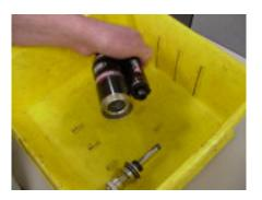
19. Under oil, screw in the damper assembly hand tight until damper cap is flush with the damper body.
