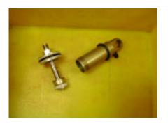
11. Under oil, install air piston/damper onto the damper body hand tight. 12. Remove from oil with damper shaft pointed up. 13. Insert needle and needle o-ring at end of damper shaft.
