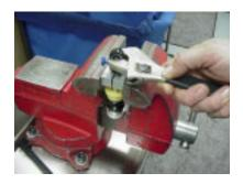
12. Using pliers, remove the rebound adjuster needle from end of the damper shaft.
