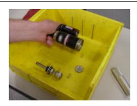
16. Under oil, insert the IFP into the air reservoir using the Swinger Air IFP removal tool. Only press the piston in just beyond the reservoir threads.
