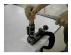
21. Holding the assembly over the oil container, Install rebound adjuster needle, pointed end first. Push until the needle oring seats in the damper shaft.
