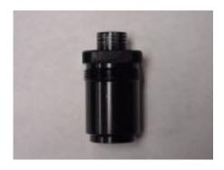
18. Under oil, screw in the IFP locating tool into the air reservoir body. This will press the IFP deeper into the reservoir body to the required depth.
