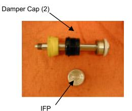
8. Reinstall IFP into the damper body. Push IFP to the location shown below based on the shock eye-to-eye and travel. Relieve any backpressure in the air preload chamber and install the Schrader valve cap. Use shock pump to move the IFP towards the damper body opening if it was inserted too deep.
