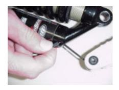
11. Remove Eyelet as shown under the section on BOTTOMOUT BUMPER REPLACEMENT
