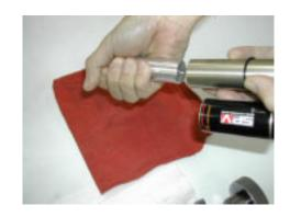
Change out o-rings and seals where indicated (#of o-rings/seals in each assembly noted in photo) and grease with a thick grease such as Motorex Bike Grease 2000
