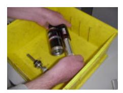
17. Using a 6mm hex wrench, adjust the IFP Locating Tool so that the indicated travel matches the shock travel.
