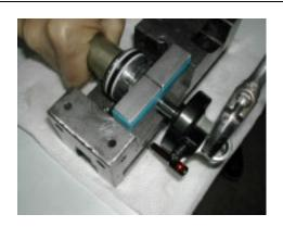
Clamp the damper body eyelet in a vise using soft jaws and remove the damper assembly by removing the air piston as shown. Remove from vise and drain damper oil into a container and discard.
