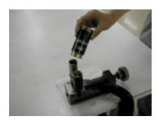
7. Remove air piston from canister
