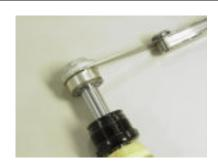
5. If it is necessary to remove the valve, clamp the damper shaft using soft jaws and loosen the damper piston bolt. Grasp the damper bolt, piston, SPV, and SPV backing plate and remove as a set from the damper shaft.
