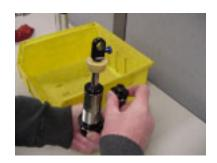
23. Apply blue loctite #242 to air preload adjuster threads and grease threads. Install the air preload adjuster and tighten to 43KgCm (50 inlbs)
