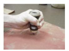
Remove IFP (Internal Floating Piston) using IFP removal tool (85-4413). Insert the removal tool into the top of the damper body. Cover hole in tool with your thumb. Point the reservoir body <u>away</u> from you and push the tool to the bottom of the damper body.
