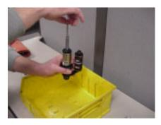
21. Install eyelet as shown under the section on BOTTOMOUT BUMPER REPLACEMENT.
