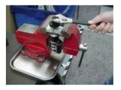
24. Remove the IFP location tool. Once the tool is removed DO NOT move the damper shaft
