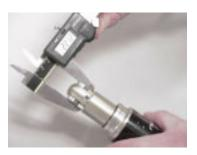
2. Measure mounting hole size. Current hardware is typically designed to accept a 6mm or 8mm fastener.
