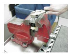
6. Remove the SPV backing plate and SPV. It is best to replace a defective valve.
