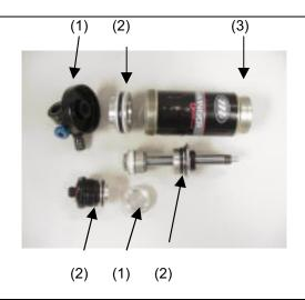
Install Air Canister Seal Guide onto damper body. Lightly grease damper body and slide air canister over body. Remove guide.
