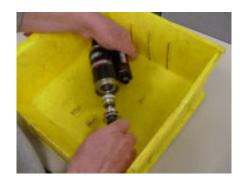
20. Remove the assembly from the oil, keeping the open end of the damper shaft pointing up. Using soft jaws to protect the eyelet, clamp the reservoir eyelet and torque the air piston per Table 1.
