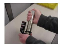
Replace external o-rings on damper cap, IFP, and air preload assembly as shown. Grease with a thick grease such as Motorex Bike Grease 2000.
