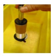
11. Holding the assembly over the oil container, Install rebound adjuster needle, pointed end first. Push until the needle oring seats in the damper shaft. Tighten damper cap.
