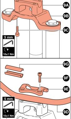
Picture 9 - Handlebar Clamp Installation
