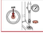
Spring preload with air - Left leg (Not present in the version with + ETA option)
