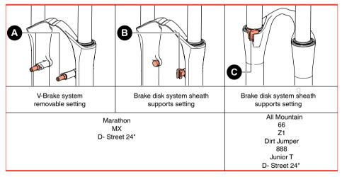
Picture 3 - Braking system settings
