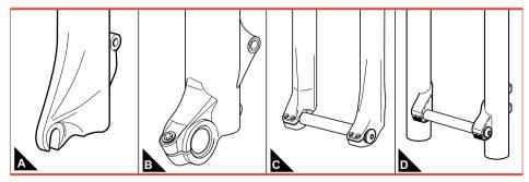
Picture 4 - Wheel securing systems: (4A) standard dropouts, (4B) ø 20mm through-hole axle (forks with ø 32mm stanchions), (4C) ø 20mm through-hole axle (66 and 888 series forks), (4D) ø 20mm through-hole axle (Monster).
