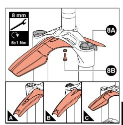
Picture 8 - Fender Installation
