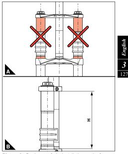
Picture 2 - Dual crown forks installation on the frame: (2A) Crowns fastening, (2B) Steer tube maximum length between crowns
