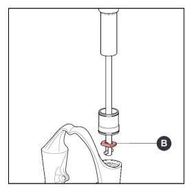
Pull the extractor rod so that the upper face of the washer stops against the lower face of the guide bush.
