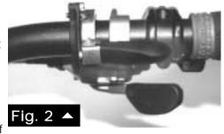
the bearings are too tight (you feel grittiness or resistance) or too loose (you feel lateral play), loosen the lockout lever set screw and use circlip pliers to loosen or tighten the inner bearing race (see Fig. 1). When the bearings are adjusted properly, reset the detent preload, tighten the lockout lever set screw, and continue with the installation.
