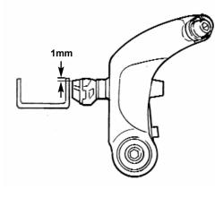
ANCHOR THE CABLE Feed the cable into the straddle wire and attach it to the brake. Pull the cable tight enough to have clearance of 2.5 - 3mm, per side, between the rim and the brake pads. Tighten the cable anchor bolt to the specified torque.
